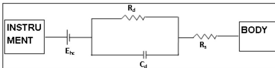
**Figure 1: Equivalent Circuit of an ECG Electrode**
