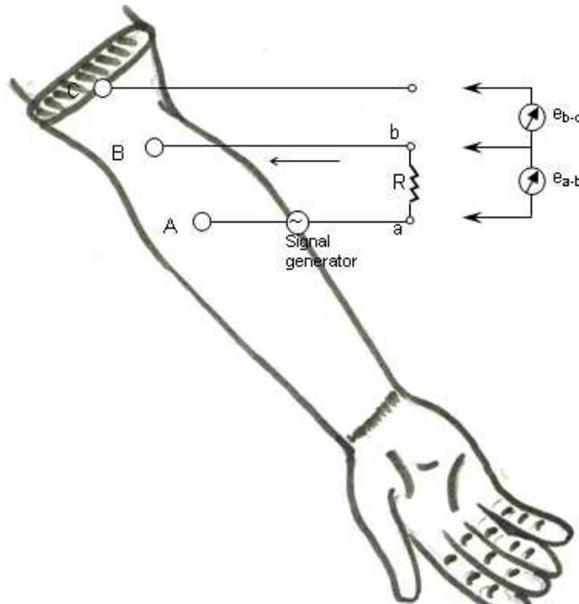
Figure 2: Arrangement for Measuring the Impedance
