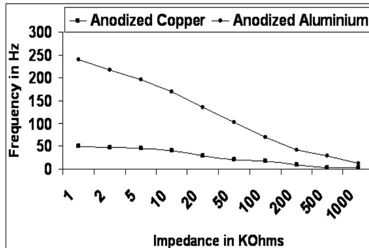
Figure 3: Impedance of the Tests Disks at Various Frequencies in the Absence of Perspiration
