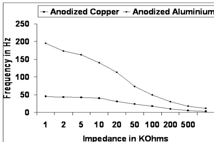
Figure 4: Impedance of the Tests Disks at Various Frequencies in the Presence of Perspiration
